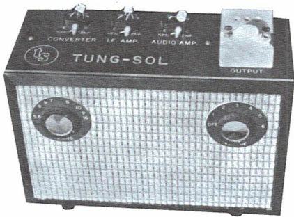
TUNG-SOL TRANSISTOR SALESMAN'S DEMONSTRATION RADIO – This AC-powered radio has switches that change polarity for PNP-NPN transistors. The left-hand dial has CD markings. ( V. Vogt – Renton, WA )
