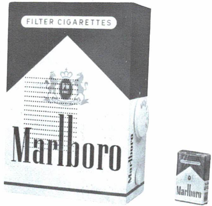
AC/DC NOVELTY RADIO MODEL UNKNOWN – This standard 5-tube AC/DC novelty radio with no markings was made in Japan. Construction is heavy foil over wood. Its 13" x 9" size dwarfs its famous cigarette pack counterpart. ( Rod Galloway – Melbourne, FL )
