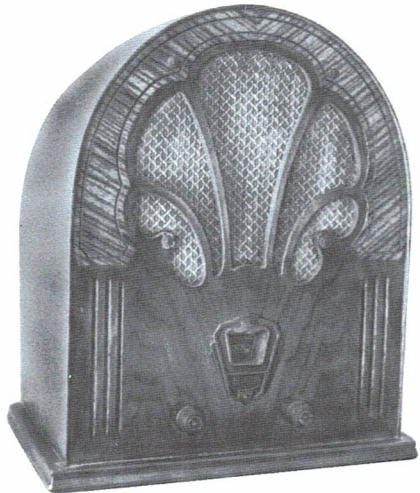
BELMONT MODEL UNKNOWN – This 5-tube set is designed to operate from the 110-volt DC mains that could be found in some of the larger cities in the 1930s. The tube complement is Type 38 (2) and Type 36 (3). The finish on the front and the grille cloth are original. The chassis has been restored and the set plays quite well. ( Bill Harris – Roanoke, TX )
