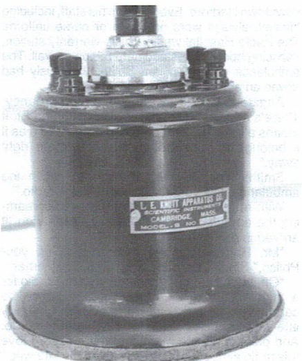
Figure 4. The driver unit of the Knott Dynamic Model B horn speaker.
