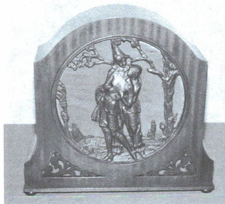
This Old Equipment contest entry by John DeLoria is a Pathe wooden cone speaker labeled "Safar." It is 20"h x 20"w x 7"d and has a solid bronze driver and grille.
