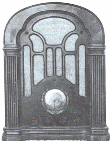
ATWATER-KENT MODEL 135-Z – Found on the "junk wagon" at a local farm auction, this all-original Superheterodyne needed only a filter capacitor to get it in working order. ( Bart Rydzinski – Winchester, IN )
