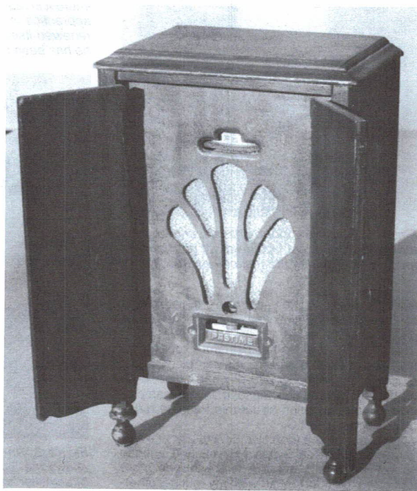
Figure 3. Note the name "Pastime" stamped into the escutcheon, the sliding on/off switch and volume control, and the thumb dial above the speaker grille.
