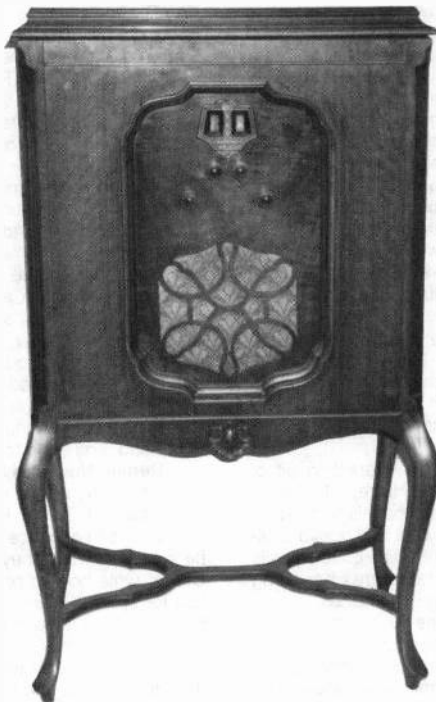
Figure 1. The E.H. Scott Allwave Superheterodyne in an early Warrington console, the top of which lifts up to expose the tuner chassis.
