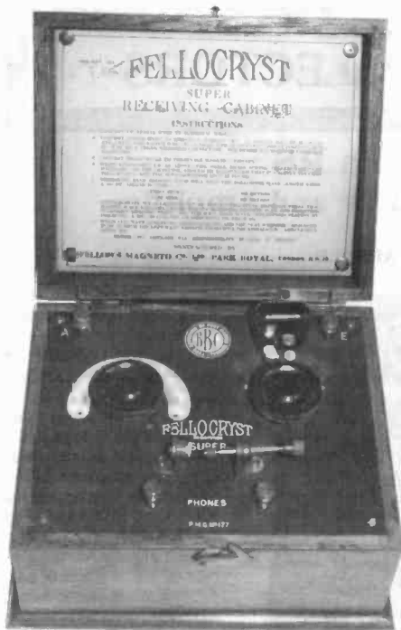
Figure 2. The Fellocryst Super crystal set.
