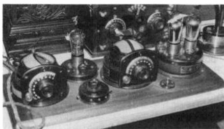
A refinished Atwater Kent open type Model 9 breadboard that was offered in the auction.
