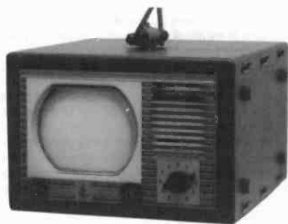
EMERSON MODEL 600 – This 1949 portable TV was in a leatherette covered cabinet. The carrying case handle is on the left side. The set uses 19 tubes and has a 7-inch picture tube. (Tony and Lynn DeMara – Mt. Clemens, MI)
