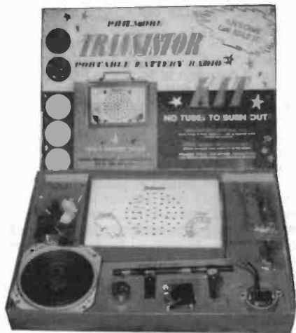
PHILMORE TRANSISTOR PORTABLE BATTERY RADIO KIT – This assembled kit uses 2 transistors listed as PH3 (TR1) and PH2 (TR2) plus an IN34 Germanium diode (D1). It tunes from 550 to 2500 Kc. (Michael Crain – Harveys Lake, PA)
