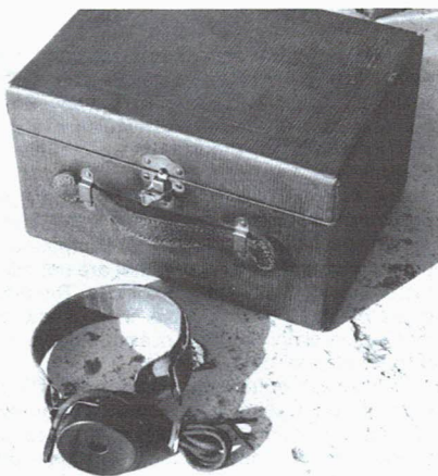
Figure 1. The AC Companion in its leatherette box and single leather band headphone.
