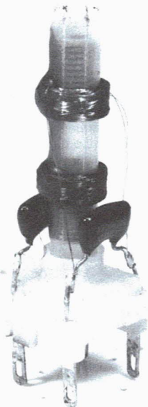
Figure 9. Zenith transformer after rebuilding.
