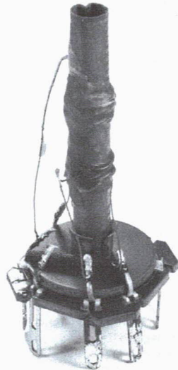
Figure 10. Zenith large footprint FM discriminator transformer with the cover removed and the wires removed from the pins.
