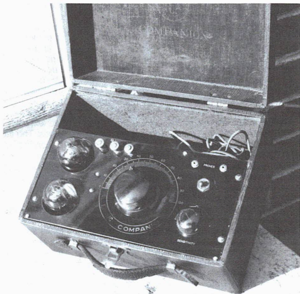
Figure 2. The AC Companion with the cover open. The power cord can be seen in the storage compartment.
