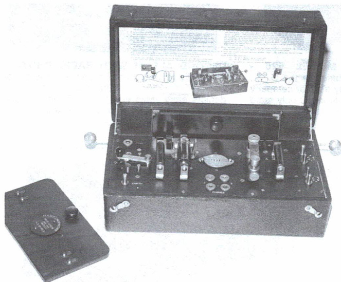
Figure 1. Marconiphone RB10 receiver with lid open and spare range block.
