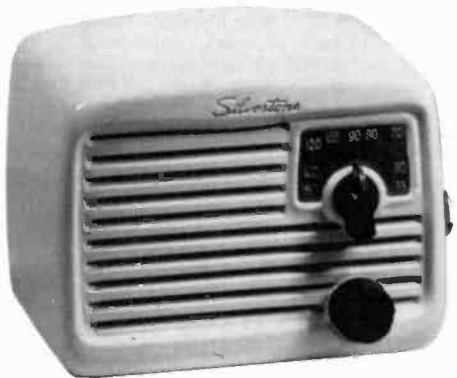
SILVERTONE MODEL 132-018 - A metal cabinet painted ivory with a maroon dial and red lettering made this 4-tube superhet AC/DC set a real buy in 1946. (Fred Geer - Jacksonville, FL)
