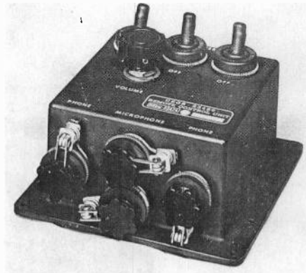
Figure 7. Waterproof remote control switch box with special spring bands around the rubber to prevent water entrance.
