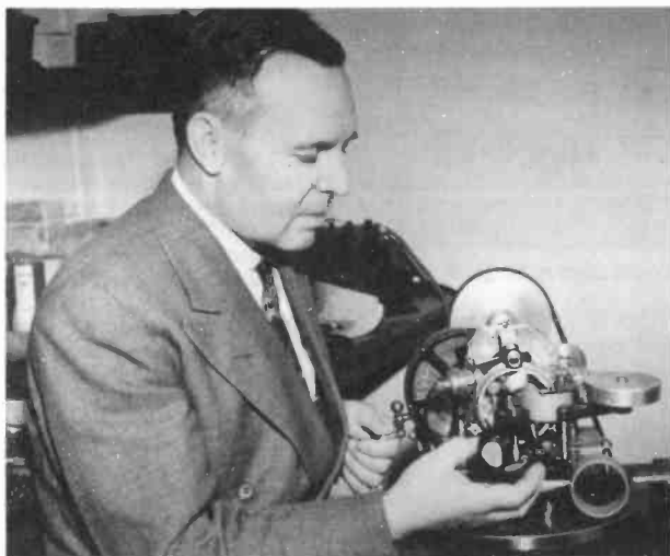
Figure 8. R.R. Gonsett with his toroid coil winder, now on display in the museum of the University of Alberta, Canada.
