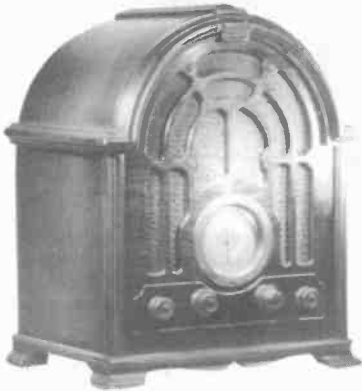
RCA VICTOR MODEL 121 - Built in 1932, this is one of the most impressive RCA cathedrals. The band selector is a pull switch. Unlike so many RCA models of the early 1930s, the chassis on this model is more accessible. (Fred Geer - Jacksonville, FL)
