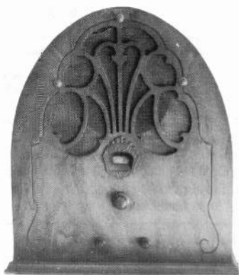
PHILCO MODEL 20 - Also known as the "Baby Grand," this AC-operated TRF set, made in 1930, was Philco's first cathedral radio. It uses seven tubes and covers the broadcast band. (Ron Ramirez - Providence, KY)
