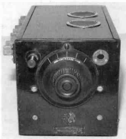
Figure 2. View showing the controls of the Western Electric power amplifier.
