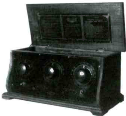
KARDONSTRIP - This 1925-26 five-tube TRF receiver was made in New York City by the Kardon Radio Corp. Manufacturer Peter Kardon designed and patented the novel "strip" wiring method, consisting of bronze strips eyeleted to the Bakelite sub-panel, which also served as tube socket connections. This battery set retailed for $35 with production cost at $7 to $10 each. I would like to know of the cabinet manufacturer, as this cabinet was also used by Leutz and others. (Mike Parker - Portland, OR)
