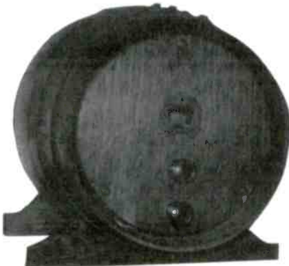
R. K. RADIO LABORATORY RADIOKEG - An unusual novelty radio made in 1934, this keg is made of oak with copper barrel straps. The speaker and a small copper spigot are on the rear of the set. (David & Terry Masterson - Cheshire, CT)
