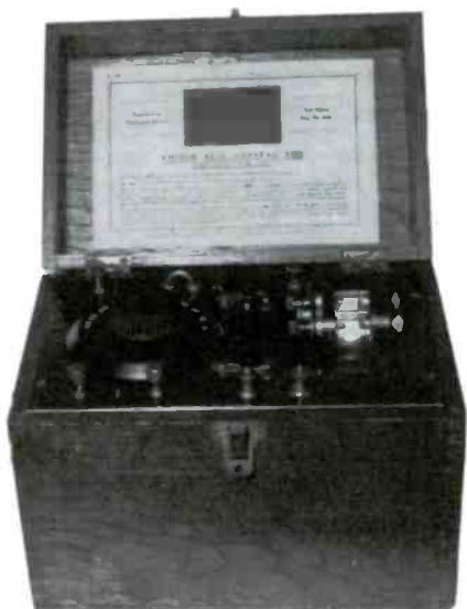
EDISON BELL CRYSTAL SET - This rare set was manufactured by Edison Bell Ltd. in 1923. The crystal detector is illuminated from below by a small bulb. The Government Post Office (GPO) Registration is No. 615. (Erwin Macho - Vienna, Austria)
