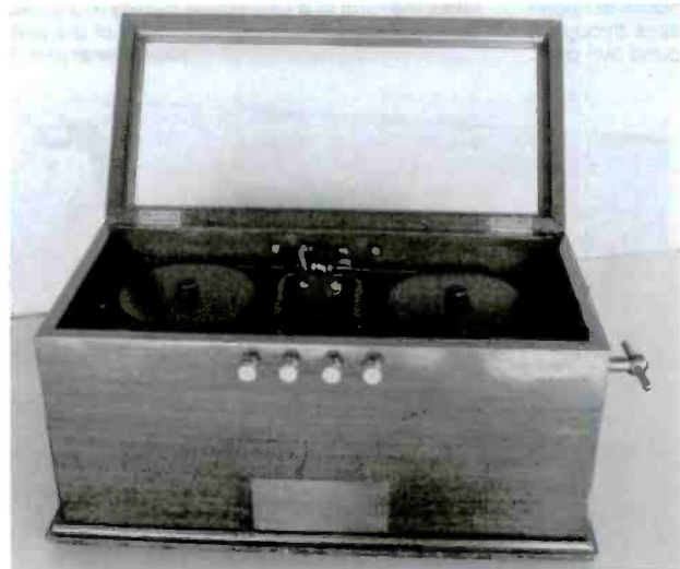
Figure 5. The Marconi Magnetic Detector was less sensitive than a Carborundum or crystal detector but was more rugged and therefore desirable for shipboard use. Because of this, it continued to be used long after more sensitive detectors were developed. This is a very rare piece in the collector market today.
