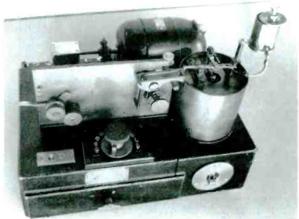
Figure 9. Marconi High-speed Recorder and Inker. Another pre-World War I device, a recorder/inker simply senses the dots and dashes of a spark transmission and converts them into a printed record by placing ink trails on a moving paper tape.
