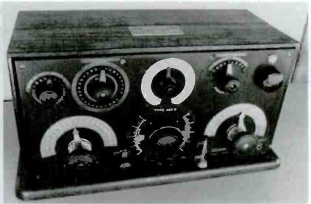
Figure 12. Marconi Model 106-D Receiver. The 106-D was a modified version of the 106-B and 106-C using a vacuum tube detector.
