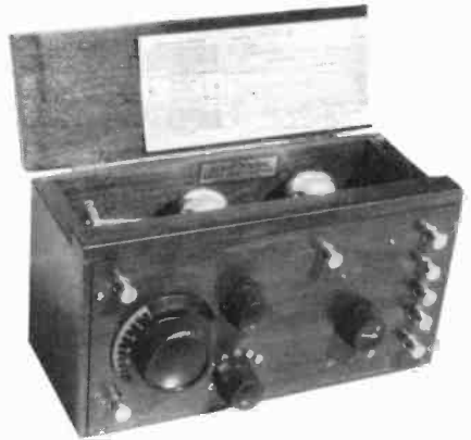
UNIQUE CROSLY - This Crosley Model 51 has a front panel made of wood! The lettering is stamped in the same configuration as the standard later version Model 51. Like most Crosleys of this era, it is regenerative with two tubes. It was bought at an auction in the original box and was never used! (Augie Walackas - Whitman, MA)
