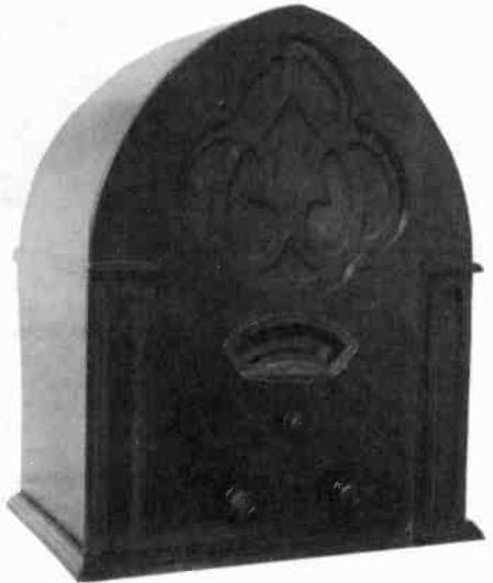
STROMBURG CATHEDRAL - This is a receiver I bought at a flea market. The name on the escutcheon is spelled "Stromburg" (not to be confused with Stromberg-Carlson). A "Phono Home Broadcast" plug is mounted on the rear. There is no visible model number or other information about the manufacturer on the set. This five-tube TRF receiver uses tube Types 80, 47, 57 and two 58s. (Richard L. Bednarcik - Lincoln Park, NJ)
