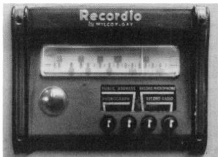
Figure 6. Model 6B30 radio dial and selection switch. (No full shot of this one as the cabinet is in the process of being restored, and the turntable is not installed.)
