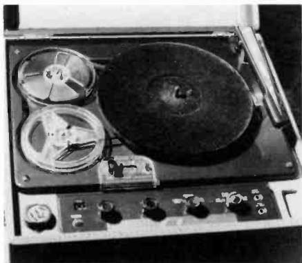
Figure 4. Model 1C10 with built-in tape recorder and disc recorder, no radio, 78 speed only. Same tone arm used for both cutting and playing by changing needles.
