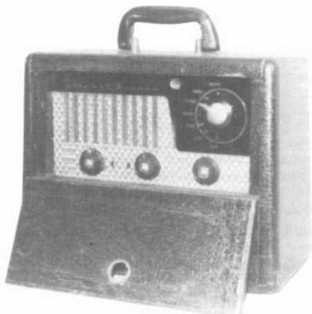
THREE-WAY PORTABLE - The Stewart Warner Mocol A61P1 is a six-tube, three-way portable with built-in battery charger. Manufactured in 1947, this radio has a black leatherette-covered case and a handle that looks like that of a Zenith Trans-Oceanic. (Walter Worth - Wollaston, MA)
