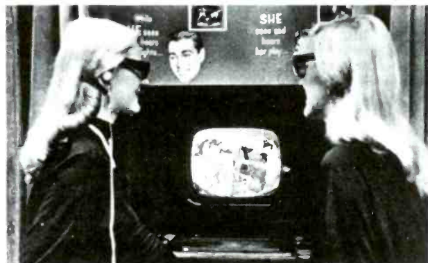
Figure 1. Twins wearing polarized glasses and separate hearing devices, watching different television programs on the same screen.
