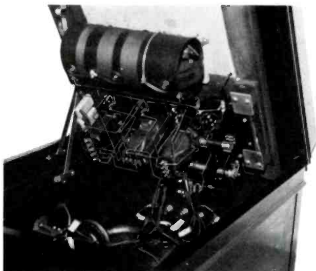
Figure 5. The circuitry and wiring of the Radiola Grand mounted under the panel.
