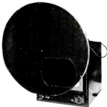
Early color television set with a spinning color wheel, a contest entry.
