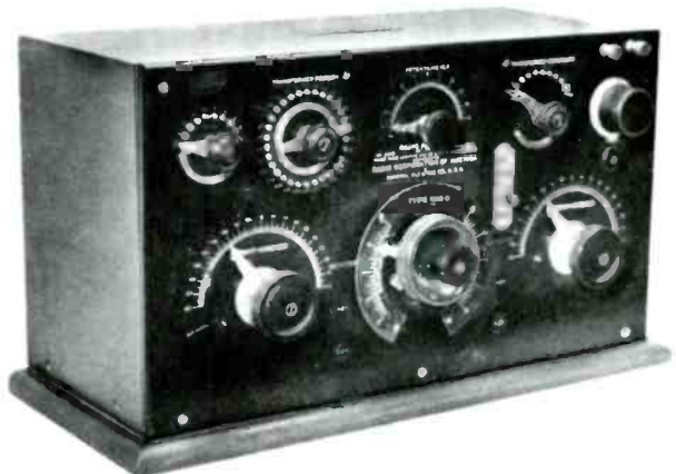
Figure 2. The author's restored Marconi Model 106D Receiver converted from a Type 106B. [Figure 1 shows correct knobs and buzzer cover; restoration is still underway on the author's set.]
