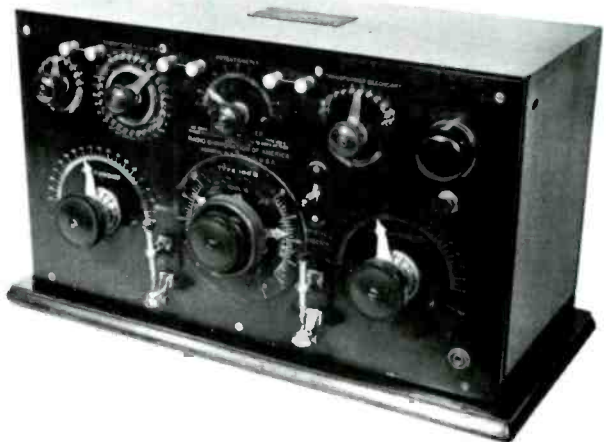
Figure 1. The RCA Type 106D Receiver modified from the Type 106C by General Electric Co. showing the two crystal detector units still in place. (From the collection of John V. Terrey.)
