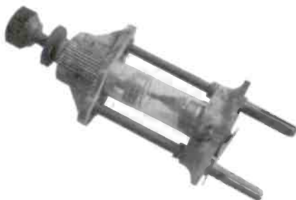
GERMAN DETECTOR - This "Radlif Detektor" (crystal detector) was manufactured by John Lifschitz of Vienna in 1927. It has a brush-type cats whisker enclosed in a glass cylinder. (Erwin Macho - Vienna, Austria)
