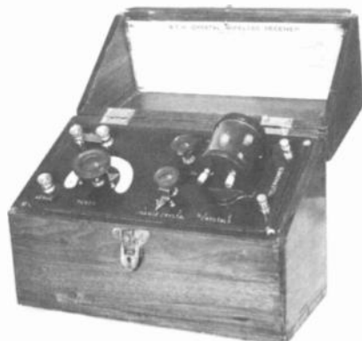
Figure 3. Model A. G.P.O. #0373. It was manufactured by the British Thomsom-Houston Co., Crown House, Aldwych, London. The date was 1922. It is in a walnut case with lid and sloping panel inside. It is 5 1/4" x 8 1/4" x 11 1/4". It has variometer tuning, and for £0.3.6 extra, a loading coil be purchased. It cost £7.15.0. It is an excellent performing set.
