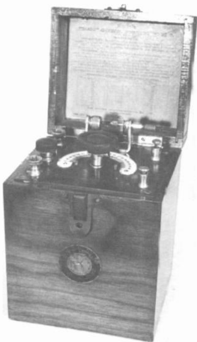
Figure 4. Bijou. G.P.O. 861. It was manufactured by the British Thomson-Houston Co., Crown House, Aldwych, London. It first came out in 1923. It has a walnut case with a lid. It is 4\frac{3}{4}'' \times 5\frac{1}{4}'' \times 7\frac{1}{4}'' . It uses variometer tuning. It cost £3.10.0 including a set of headphones. A 5XX loading coil was £0 3.6 extra. It is a very well made set.
