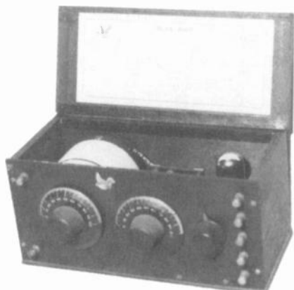
BLUE BIRD - This tube set of the early 20's was manufactured by the Automatic Radio Company of Boston. It has bakelite paneling and is in a leatherette-covered wood case. The TRF design has no regeneration. Note the bluebird on panel. (Walter V. Worth - Wollaston, MA)
