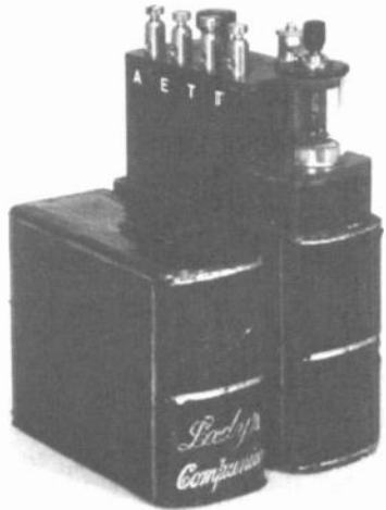
Figure 6. The Lady's Companion. This is a home-built crystal set of very fine craftsmanship. The case is red leather with gold lettering. It has an enclosed glass crystal detector. It is tuned by moving the lever in and out. The date is circa early 1930's. It is quite small, 3\frac{1}{2}'' \times 2\frac{1}{4}'' \times 1'' .
