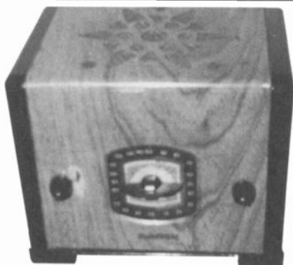
CLINTON RADIO MFG. - This all metal radio has a light green wood grain front and top and black sides. It was manufactured in Chicago, Illinois, ca. 1936. The BC/SW dial has several different colors. The radio features 6 tubes, with the speaker mounted in the top. (Jimmy Downes - Covington, LA)
