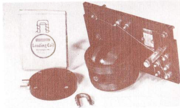
Gecophone No. 1. Interior view, loading coil and loading coil bridge.
