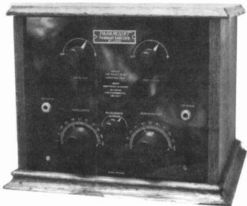
PARAMOUNT - Actually a Echophone Type "A" manufactured by The Radio Shop of Sunnyvale, California. It is a three tube set using the Armstrong Patent for regeneration. (Greg Farmer - Fridley, MN)
