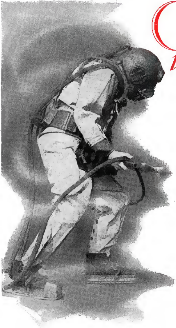
This illustration is a reproduction of a photograph of Commander Edward Ellsberg in a diving rig with an air drill rigged for underwater use (Description dictated by Commander Ellsberg)
