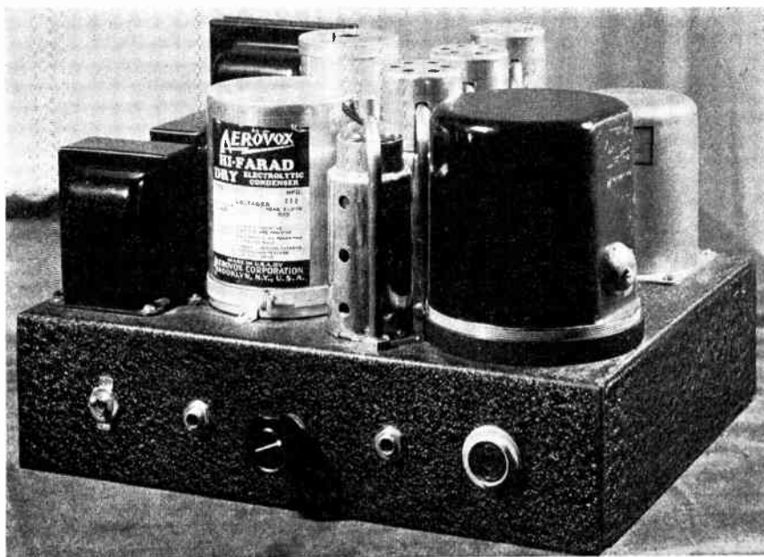
Front view of chassis. Note the method of shielding grid leads as shown in first tube with shield can cap removed.
