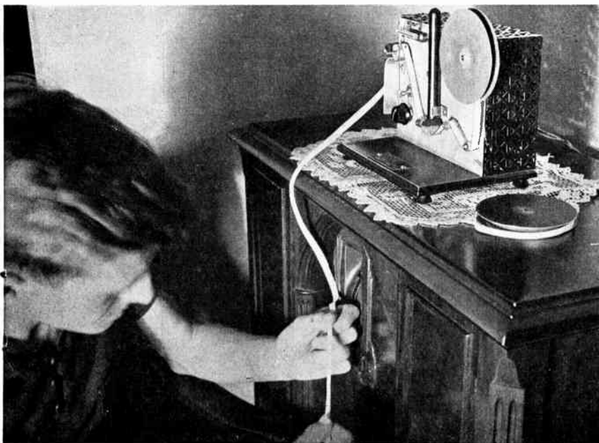
The code recorder operating from the output of a radio receiver. Dots and dashes are recorded on a chemically-treated paper tape.
