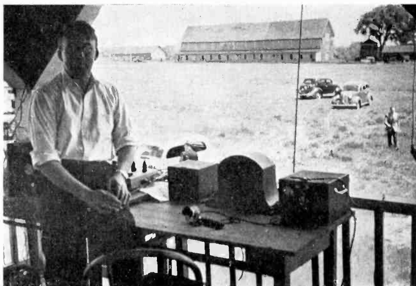
The installation on the judges' stand. Note hand mike and rod antenna.
