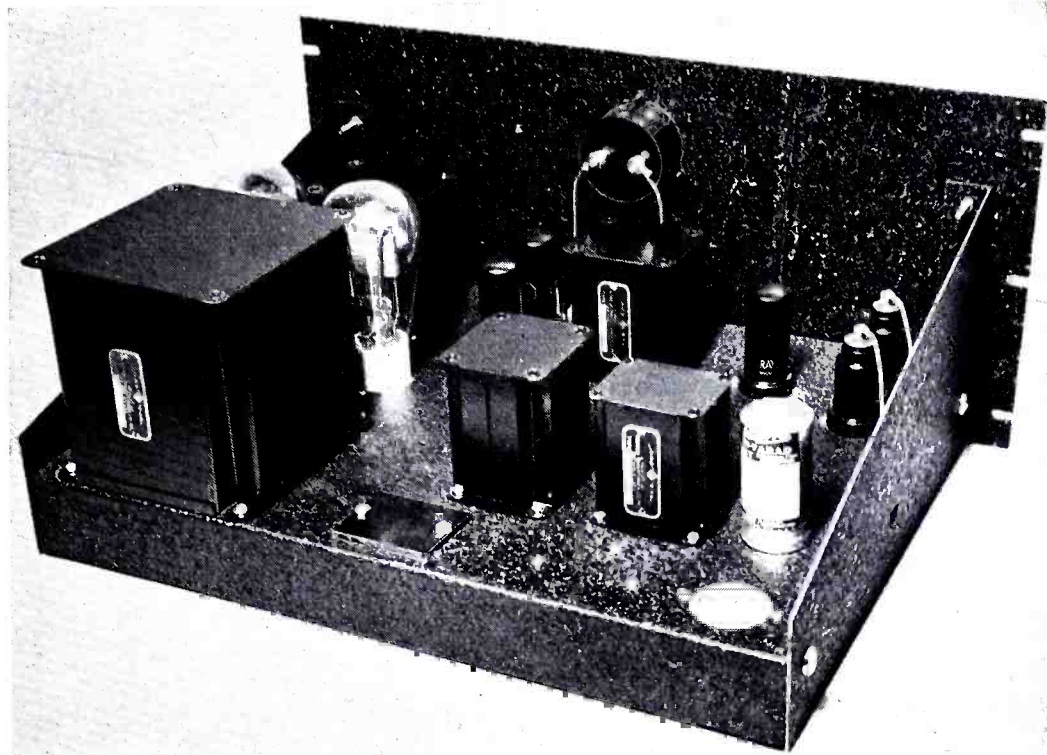
Rear view of the modulator chassis which includes the speech amplifier as well as the push-pull 756's. This is the center unit in the cabinet, as may be seen below.
