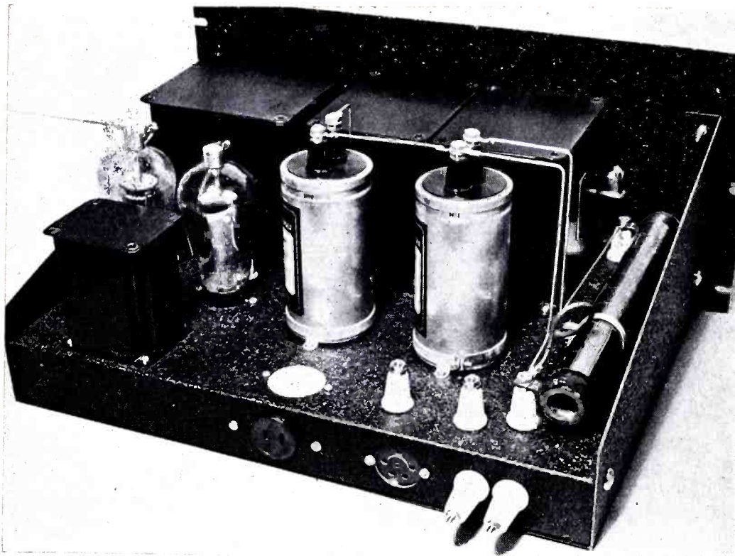
Rear view of the high-voltage power-supply chassis which employs two 866 half-wave rectifiers in full-wave connection.
