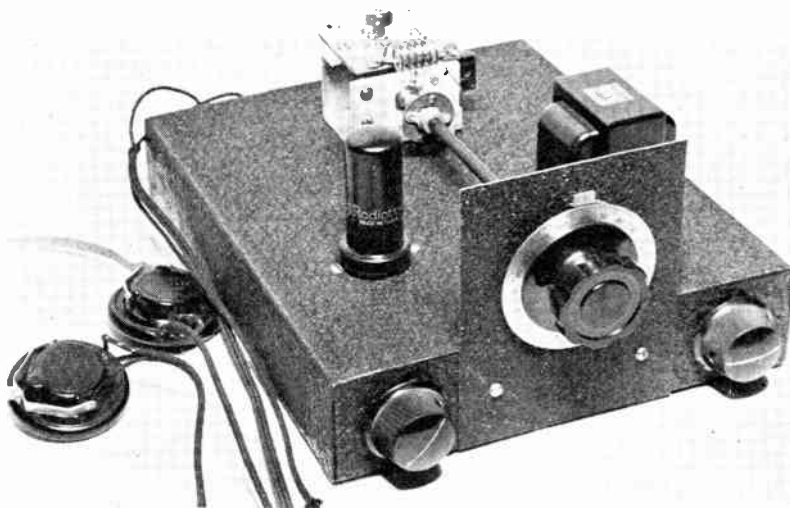
The receiving unit of the "Ground Hog." This uses a type 955 acorn tube in a super-regenerative circuit.
