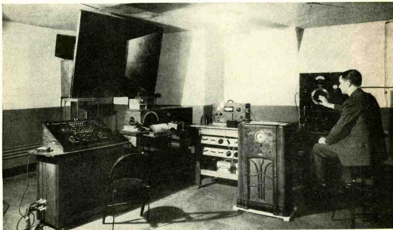
Testing radio receivers for distortion at the RCA License Laboratory. Special equipment for checking tonal fidelity is used.
