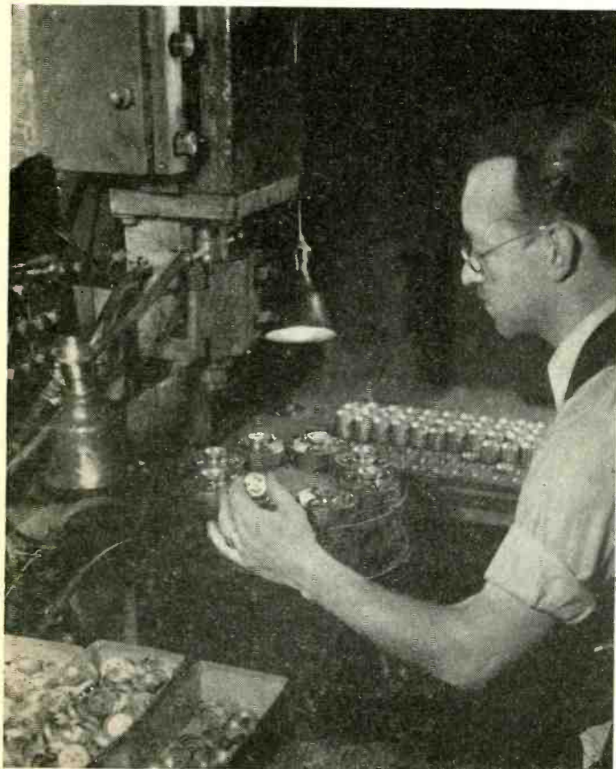
Operator welding the Fernico eyelets to the "headers" or bases of metal tubes. This operation takes but a fraction of a second.
