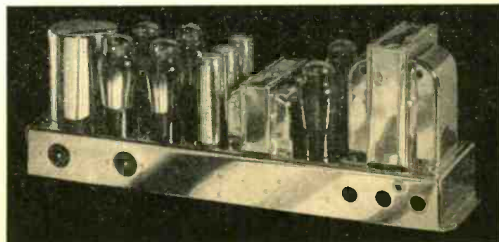
A view of the separate power amplifier of the Scott Imperial Allwave receiver.
