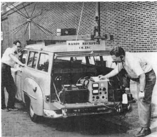
Below: Radio Receptor Co.'s mobile field unit is designed to make precise field interference measurement to determine compliance with Section 18 of F.C.C. regulations.
