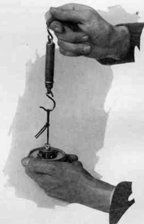
FIG. 171. TESTING MAGNET STRENGTH, HORN TYPE UNIT.
