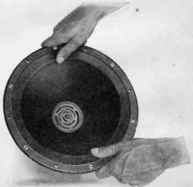
FIG. 180. TESTING TO DETERMINE IF DIAPHRAGM COIL SCRAPES ON POLE-PIECES.
