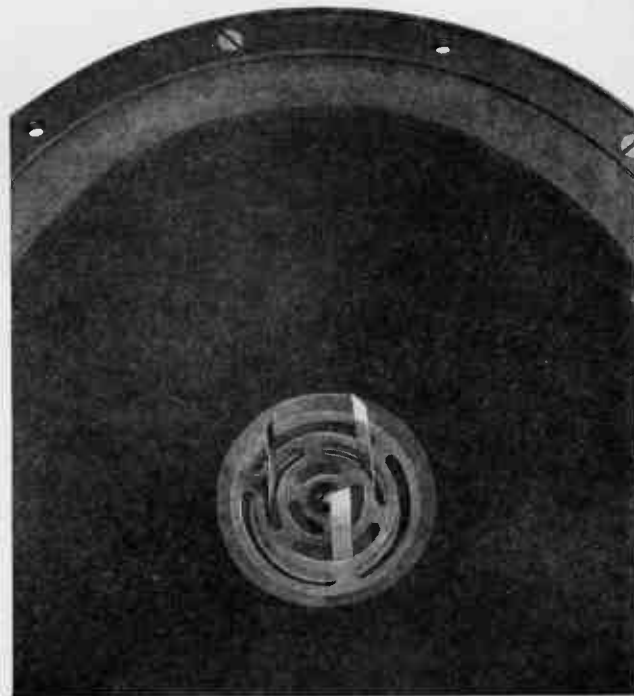
FIG. 178. CORRECT POSITION OF SHIMS USED IN CENTERING DIAPHRAGM COIL.
