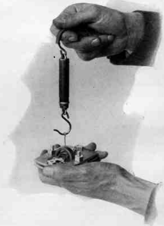
FIG. 175. TESTING MAGNET STRENGTH, CONE TYPE UNIT.
