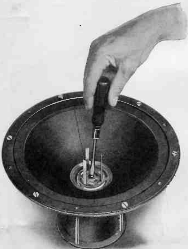
FIG. 179. TIGHTENING ROUND-HEAD DIAPHRAGM SCREW, AFTER DIAPHRAGM COIL HAS BEEN PROPERLY CENTERED.
