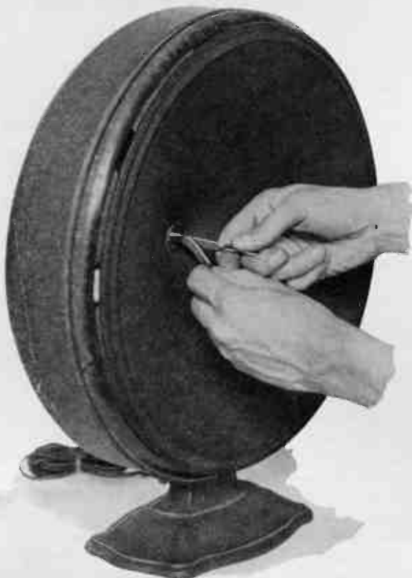
FIG. 174. REMOVING CONE, MODEL E, AND E-2.
