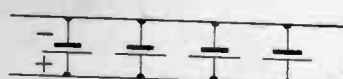
BATTERIES IN PARALLEL. The total voltage is the voltage of one branch.
