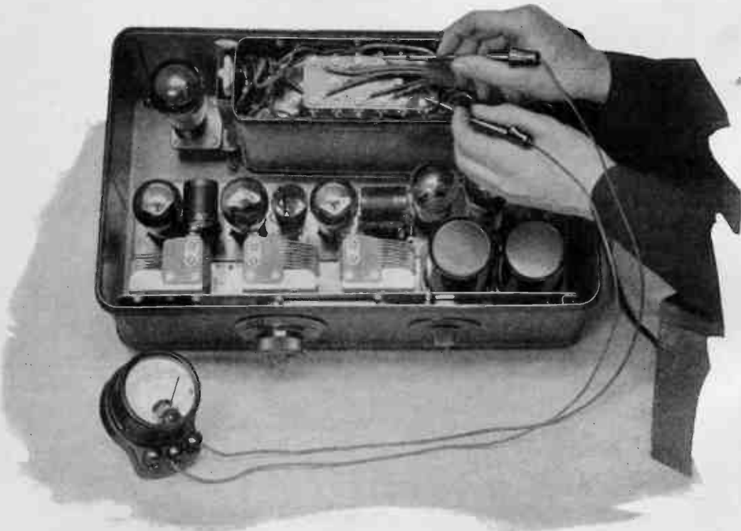
FIG. 42-A. MEASURING THE +B DETECTOR VOLTAGE AT THE POWER-UNIT TERMINALS.
