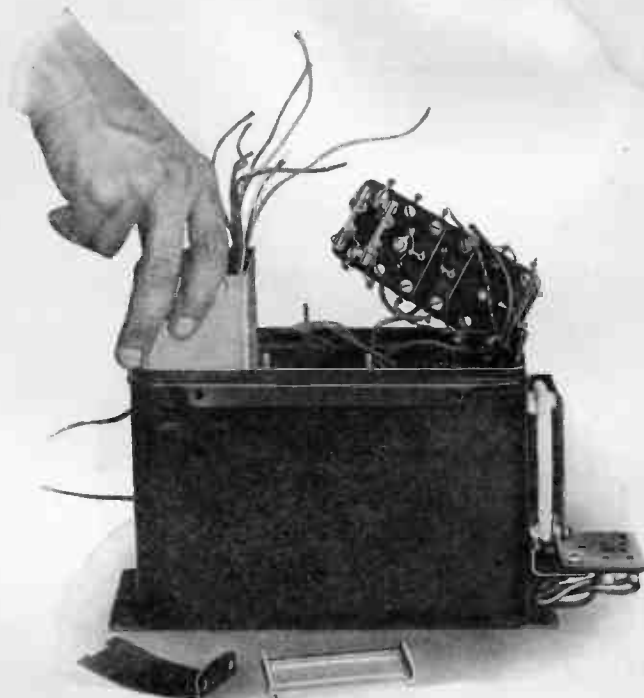
FIG. 84. REMOVING CONDENSER SECTION IN POWER UNIT FOR MODEL 40-F, 42-F, 44-F AND 2ND TYPE OF MODEL 44.
