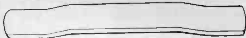
FIG. 165. VIEW OF JIG FOR SETTING COLLAR OF SLIDER AT CORRECT POSITION ON CONTROL SHAFT. The concaved or hollow side of the jig is placed facing toward the volume control. The jig is Part No. 15115.
