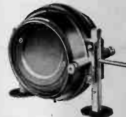
VARIOMETER The movable coil is the rotor, and the stationary coil is the stator.
