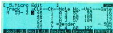
While sequencing you can change the length or dynamic value of any note simply by using microscope editing.
