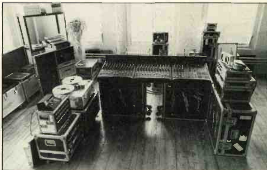
Effanel's compact cockpit needs little set-up space, travels on the same truck with the band's gear and costs half the usual remote rates.
