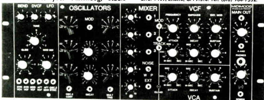
Studio Electronics' MIDIMoog modification turns the classic Minimoog into a rackmount MIDI synth module.
