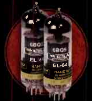
Dyna-Watt™ EL-84 Power offers two choices for wattage/wiring configuration per channel: 25w Pentode for bold headroom or 10w Triode for sweet clip-ability.
