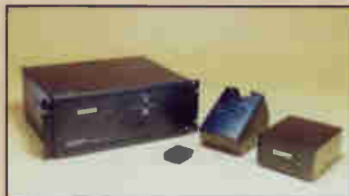
The entire PPM system (L-R): The encoder, the PPM, the docking station, and the "household hub" which collects the information from the docking stations via the household's AC wiring.
