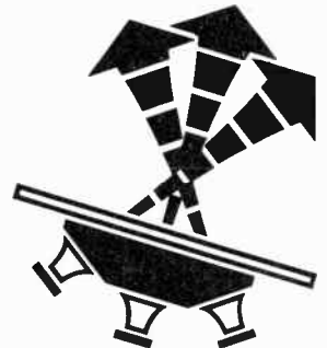
Unique "wide-angle" concave tweeter array — cuts through on-stage volume, eliminates "beaming" on-axis and muddy sound off-axis.
