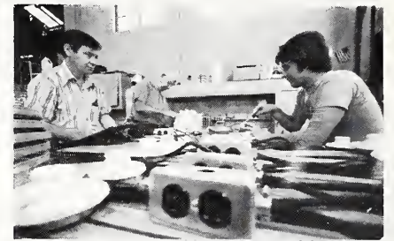
Plant technicians wiring electric lighting and signage assembly.
