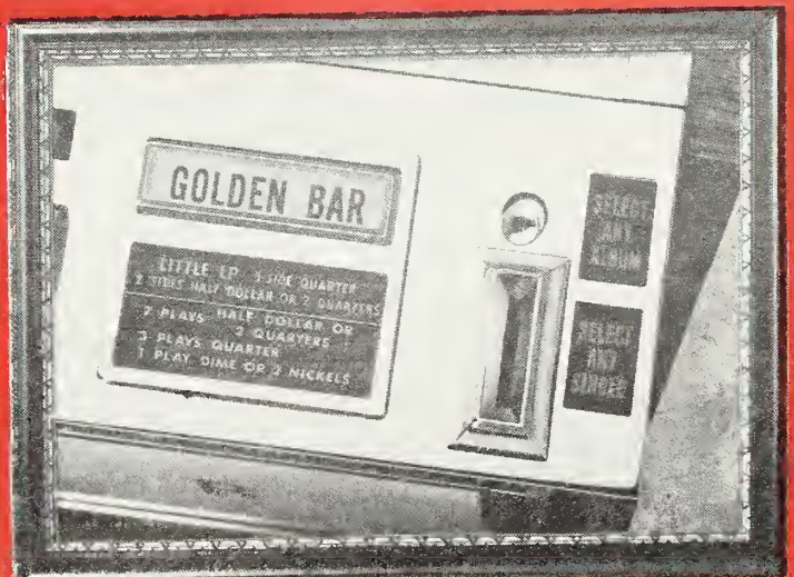
The unique Wurlitzer Golden Bar gives the patron a number of pre-selected tunes for a half dollar or two quarters. With the insertion of the required coins the Golden Bar lights up as do the two adjacent panels reading "Select Any Album" and "Select Any Single."
