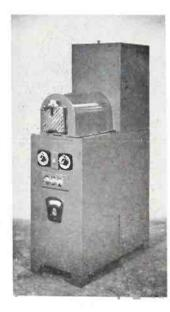
MOBILE CONSOLE TYPE, COMPACT. FAST EXTRUDER USES DRY BLEND, GRANULES, PELLETS, REGRINDS.
