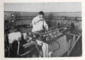
Nickel sulfamate installation for processing .010" thick finished solid nickel masters, mothers, stampers in 3-1/2 hours. Eight position—twelve position twenty position. Completely assembled. Ready to operate.
