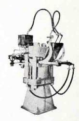
Finebilt automatic precision presses with push button automatic control. Mold closes—goes into press—mold comes out and opens. All motions are automatic. No skilled help required. One operator handles two presses.
