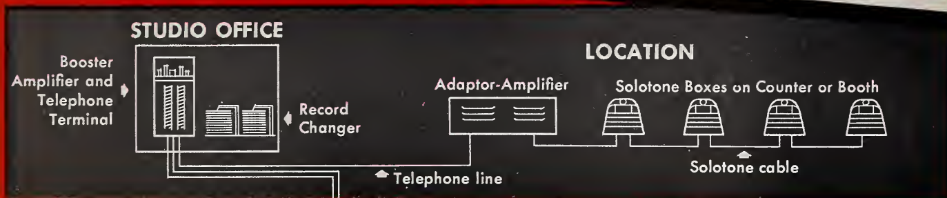
Hook-up with automatic record changer operating over telephone lines
