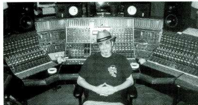
Magic Shop owner Steve Rosenthal sits at the studio's wraparound, 80's-series BBC Neve console, which features Flying Faders automation.
