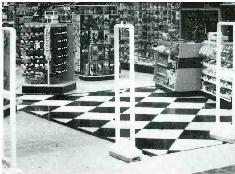
All Your Sensors Tuned. Sensormatic's microwave-based Ultra-Max EAS System is used in various types of retail locations, including music, discount, and drug stores.
