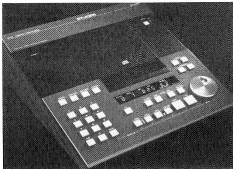
New at AES was this high-end professional CD player from Studer. The A730 is designed for on-air play and allows direct access to track and index, minutes, seconds, and frames.
