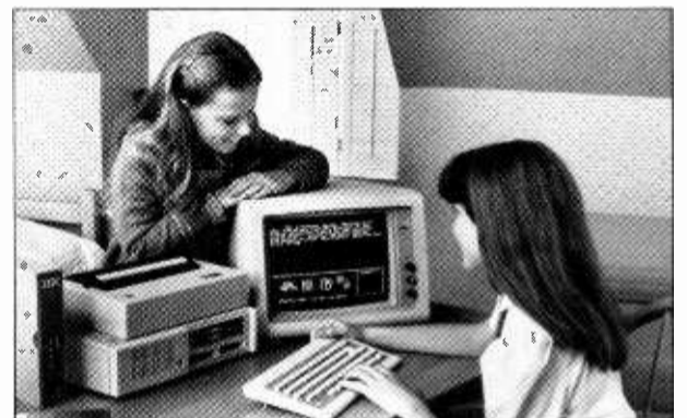
The IBM PCjr Enhanced Model includes a slim-line diskette drive, 62-key infrared keyboard and 131,072 characters of user memory.
