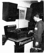
MODULAR DESIGN—A NAMM show browser tests a mix on the WR-8816 modular recording mixer from Panasonic's RAMSA division, being demonstrated here with Otari's streamlined MX5050 eightrack recorder. The mixer allows monitoring on all 16 input channels, and has two effect sends and two monitor sends, among other goodies in its "16 by 4 by 2" input/output configuration.
