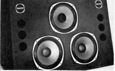
DREADNOUGHT MONITOR—This loudspeaker system from Tannoy has 1000 watts peak input, 125dB plus peak output, and is designed for large studio control rooms. A dual concentric drive unit is used. It combines an HF compression driver, and a direct radiating bass unit coaxially in a common unit.
