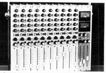
MULTI MIXER—This new model ADO62 Multimixer from Audio Developments is one of a new range of mixers with custom designed aluminum extrusions that allow for smaller, more compact systems. The unit will be on display at the AES show.
