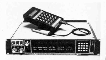
ADVANCE REVERB—This model RMX-16 is a 2U 19 inch rack mount system on an 18kHz bandwidth, offering nine programs of reverberation ranging from the smallest room to the largest hall. Once the program is selected, the user controls the delay time. Pre-reverberation delay can be added, and incependent adjustment of both high and low frequency decay characteristics is possible.
