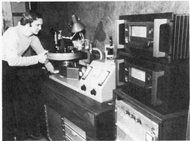
Clean Cut: Telarc Records producer Robert Woods oversees application of Threshold Stasis 1 power amplifiers as cutter-head drive electronics for the forthcoming Telarc release of Saint-Saens' Third Symphony. The mastering room at International Automated Media is the first to utilize the new amp, pictured atop the rack cabinet, right.
