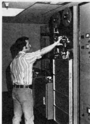
Roll 'Em: Production line operator handles one of General Cassette's high speed cassette masters.
