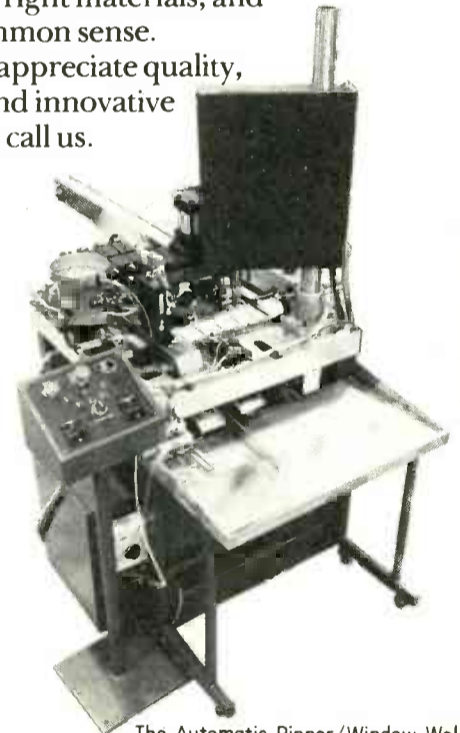
The Automatic Pinner/Window Welder designed and manufactured by Shape.
