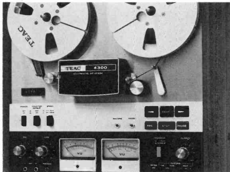
TEAC's deluxe auto-reverse play stereo, reel-to-reel tape deck at $649.50. This three motor, four head model, 4300 features 7-inch reels and records in four track two channel stereo.
