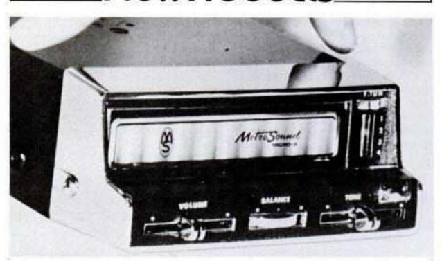
METRO SOUND claims its MS-709 Mini-Star is 'the world's smallest 8-track car stereo.' Unit features 21 watts power, slide bar for volume and tone controls, and magnetic head with automatic stop.
