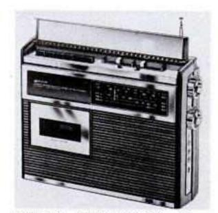
MIDLAND INTERNATIONAL, Microtron Div., released the Model 12-151 AC/DC portable cassette recorder with multiband radio and built-in condenser mike. Retailing at \$109.95, unit includes auxiliary input for recording through external phono or TV, and automatic level control to equalize near and distant sounds.
