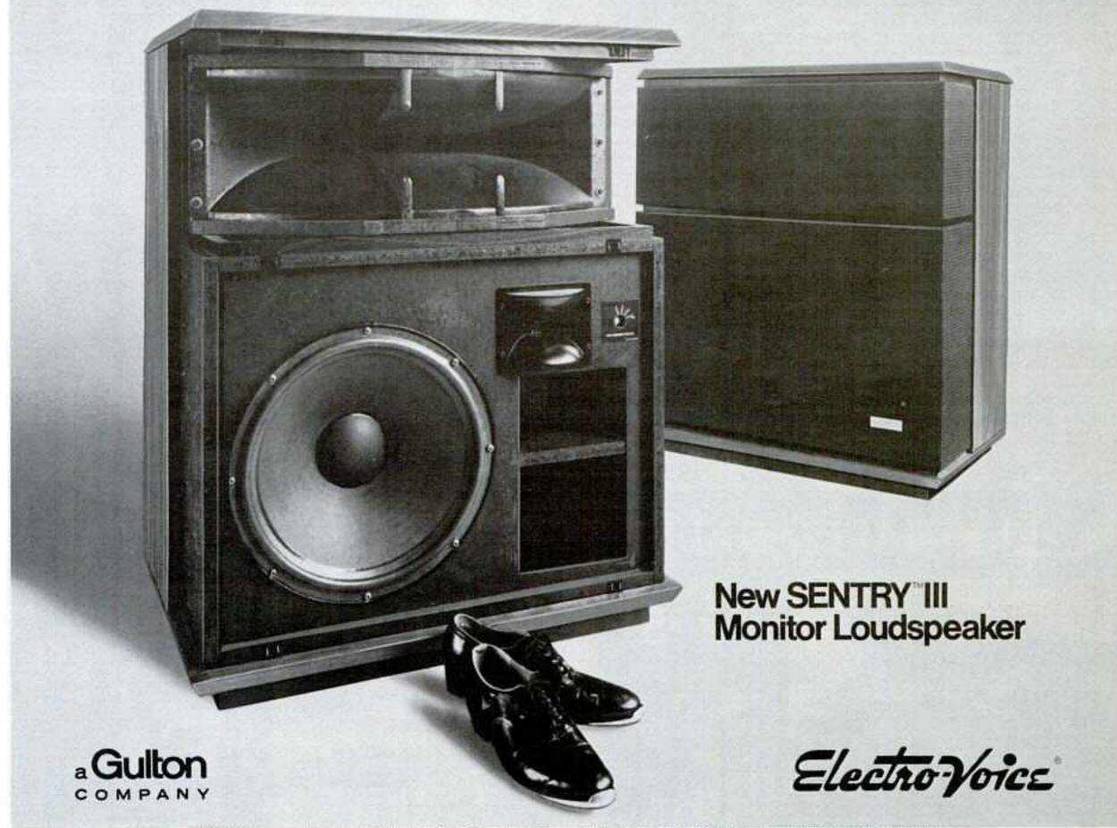
SENTRY III Frequency Response 40-18,000 Hz. ± 3 dB; Sound Pressure on Axis at 4" with 50 watt input 113 dB; Dispersion 120" horizontal, 50" vertical; Size 28½W x 20½D x 34½H; Weight 156 lbs. \$600.00 suggested professional net. SEQ active equalizer extends response to 28 Hz, \$60.00.
