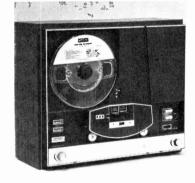
NEW VERSIONS of two new open-NEW VERSIONS of two new open-reel stereo tape recorder decks, models 1455A (pictured here) and 755A, are available from Ampex Corporation consumer equipment division. The new models, improved versions of Ampex 1455 and 755, feature improved recording and playing quality. The 1455A features in-clude sound-on-sound and echo clude sound-on-sound and echo effect. The 1455A and 755A list for \$349.95 and \$249.95 respectively.
