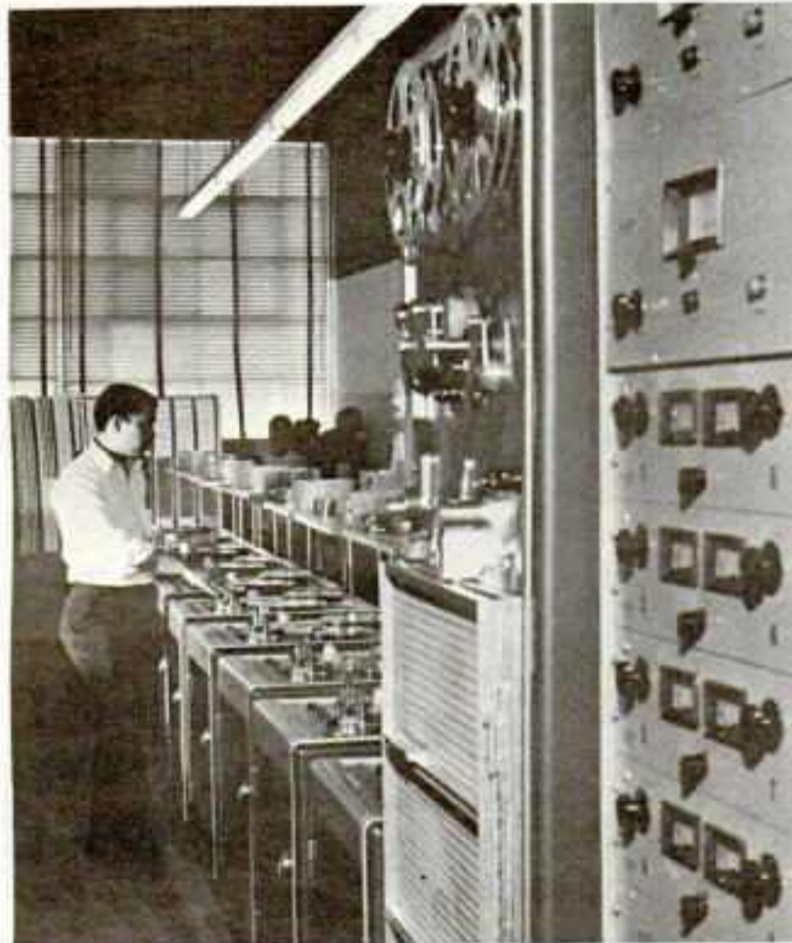
A&B Duplicators master playback rolls tape for duplication on 10 slave units. A continuous loop master unit is utilized regardless of configuration.
