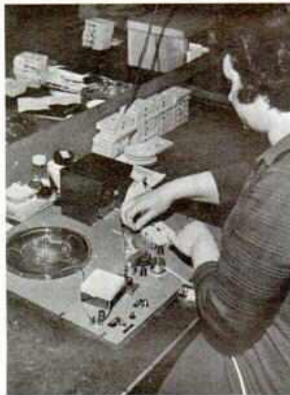
Pictured above is a closeup of the winding process as it is done on A&B's automatic unit.
