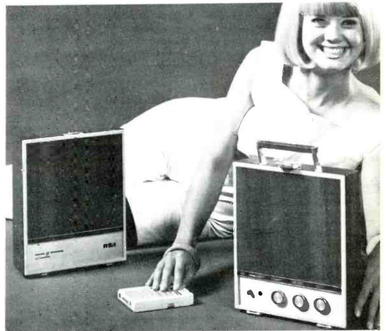
RCA'S NEW PORTABLE 8-track CARtridge player operates on batteries, house current or 12-volt source from either an automobile cigaret lighter or boat battery.
