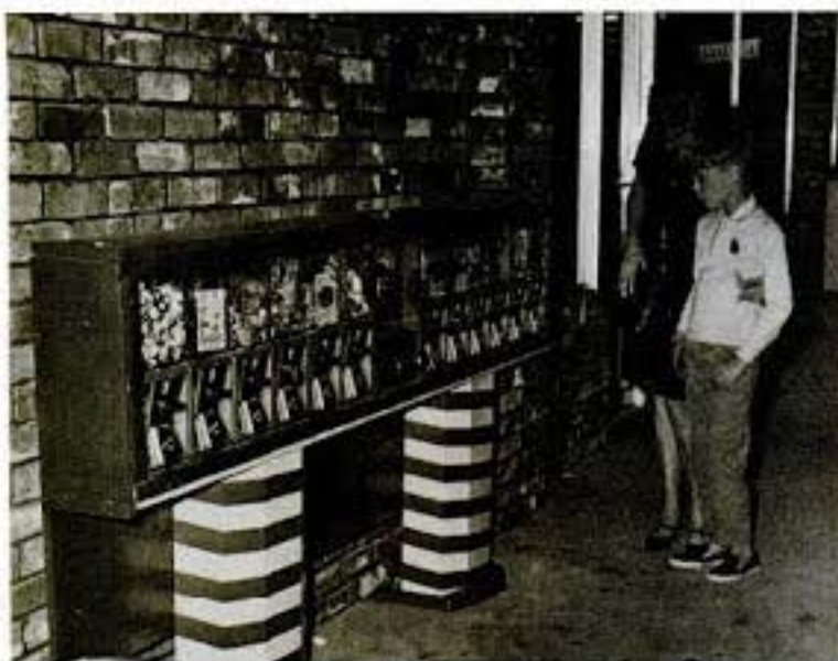
ENCLOSURE STAND designed by Dothan, Ala., operator Bert Witkos is examined outside a discount store location. The decorated supporting columns are each filled with over 200 pounds of cement.
