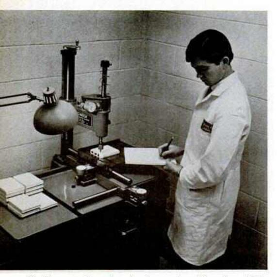
Quality control worker checks exact position of cartridge pressure roller. Machine can check other critical dimensions including cartridge thickness, location of cartridge locking detent.
