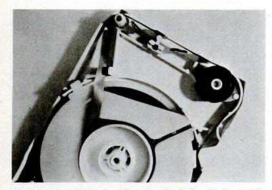
Eight-track cartridge has 13 parts of which only three—the tape, the platform on which the tape is wound and the pressure roller—move.
