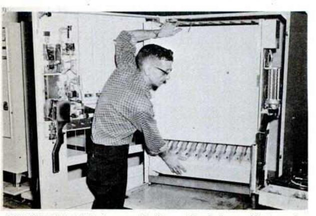
NEARING THE END of assembly line, a Candyshop cabinet receives its 10-column endless belt unit.
