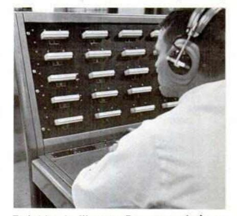
Technician in Warranty Department checks returned cartridges to verify defects using a batterytester designed and built by Record Division Engineering Laboratory. Findings enable RCA engineers to devise improved manufacturing techniques and procedures.
