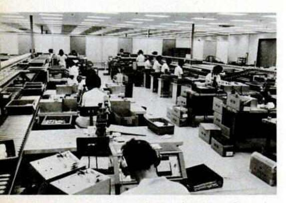
Listening tests used to confirm quality of cartridges after technical quality specifications have been met, giving finished cartridges fnal audio tests before shipping.
