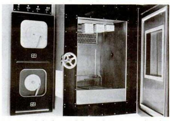
Environmental chamber in which cartridge tapes are subjected to severe temperature tests. Cartridge, its parts, and tape itself must be capable of enduring tests of temperatures ranging up to 185 degrees and down to 40 degrees below zero.
