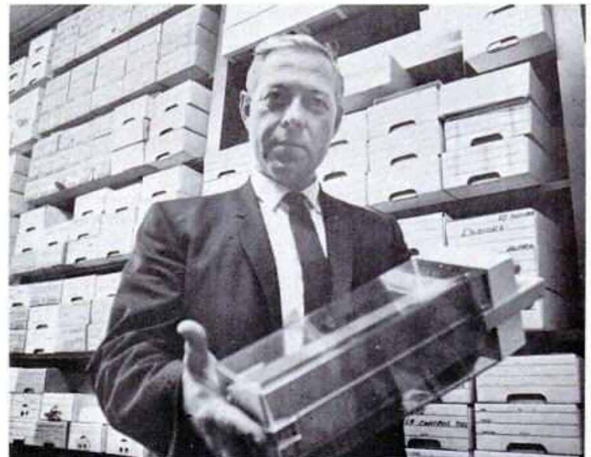
Howard Wilson holds an IBM 360 computer data cell which contains information normally stored on a half million IBM cards.
